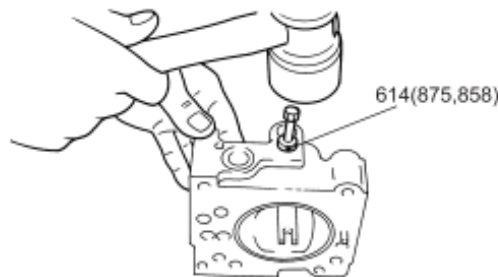
Fig. 33-128 Installing fulcrum plug (614)
