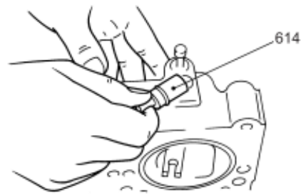
Fig. 33-118 Removing fulcrum plug (614)
