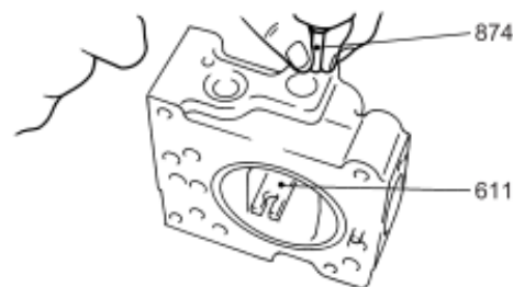
Fig. 33-120 Removing feedback lever (611) [1]
