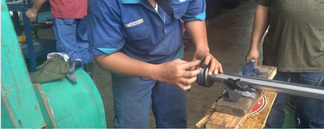
Gambar 1 Penggantian Seal Cylinder
