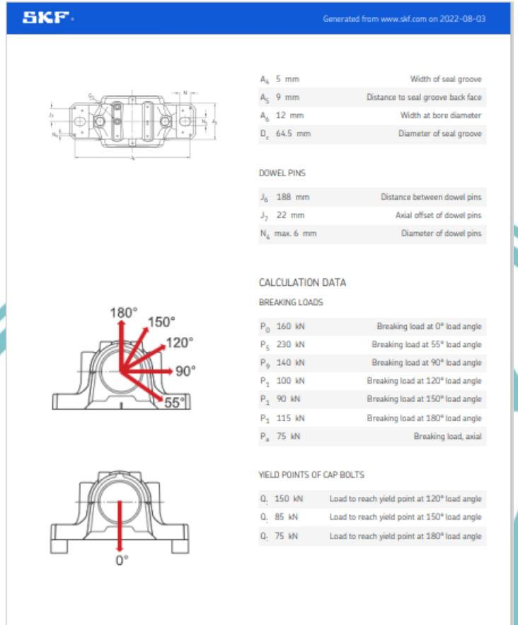
Sumber : <https://www.skf.com/group/products/mounted-bearings/bearing-housings/split-pillow-block-housings-snl-2-3-5-6-series/productid-SNL%20509>
