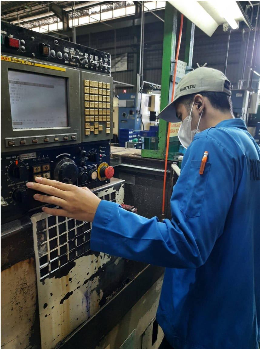
Lampiran 6. Pengecekan backlash mesin NC Lathe 1
