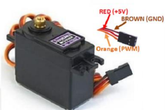
MG996R Servo Motor Wiring Diagram
