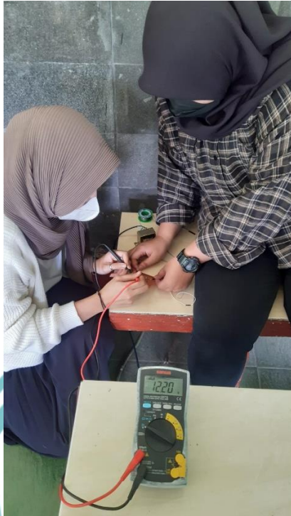
Pengukuran Output Power Supply
