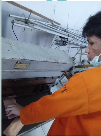
Cutting PCB Antena 1
