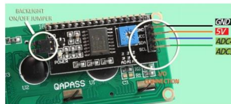
LCD display to Arduino wiring.
