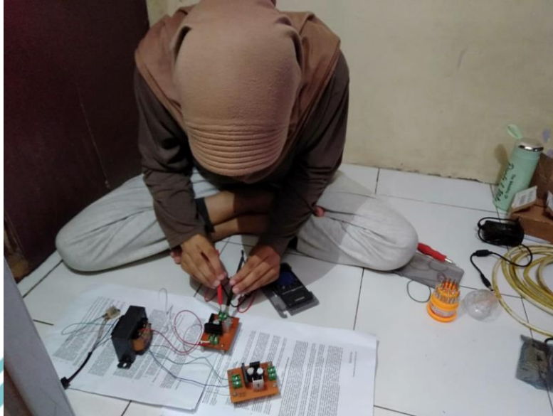
Pengujian Power Supply
