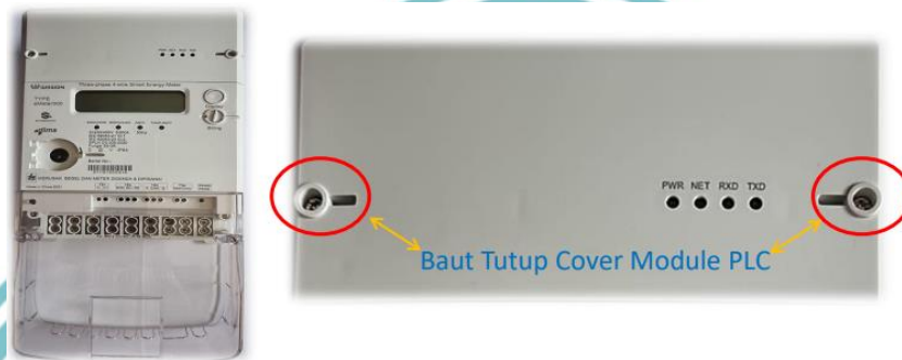
Gambar 3. 51 Tutup Cover Module PLC A aMeter 300
