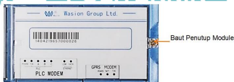
Gambar 3. 48 Master Module PLC
