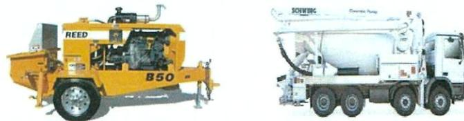
Gambar 14 . Concrete Pump
