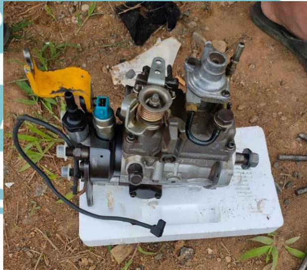
Gambar 3.24 Mencopot *Fuel Injection Pump* Dari Mesin
