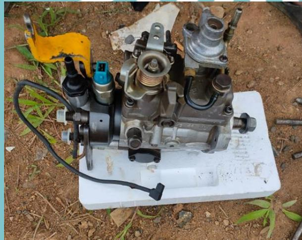
Gambar 3.11 *Bosch Pump Distributor*
