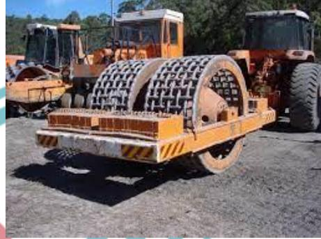
Gambar 3.3 Meshgrid Roller
