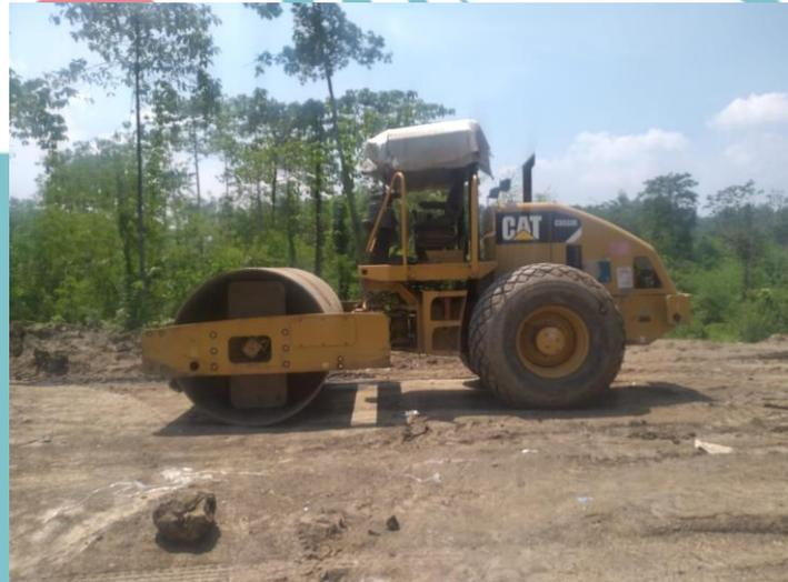
Gambar 3.7 *Vibration Roller*
