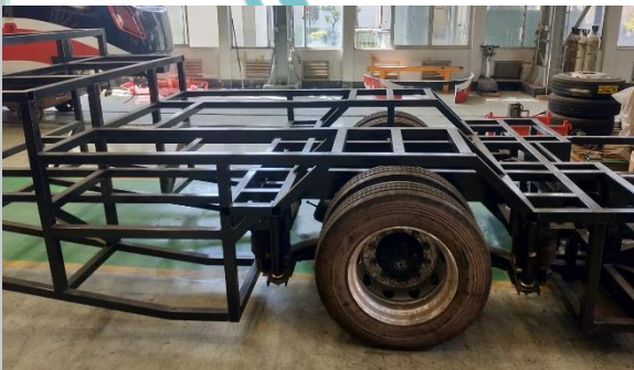
Gambar Lampiran 9 Bagian Frame Driven Axle for Rear Axle
