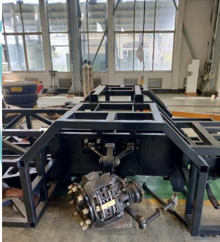
Gambar Lampiran 7 Bagian Bagian Frame Independent Front Axle
