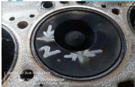
Detail piston cyl.no.2 (crack)
