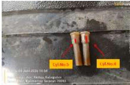
Perbedaan oil jet cyl.No 5 & Cyl.No 4(ada bekas press)
