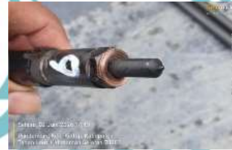
Detail condition injector no.6 (carbon)
