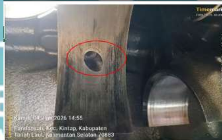
Condition actual Oil Jet Cylinder No.4 on seat (fully install)
