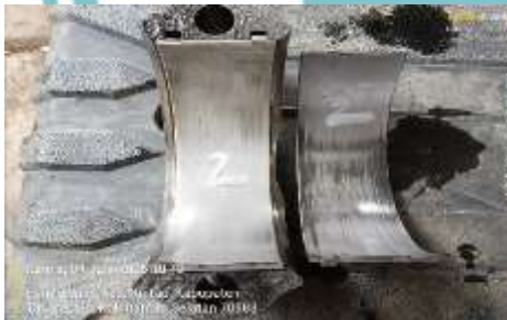
main cap bearing no.2 scratch
