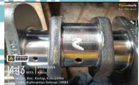
Condition Crankshaft cyl.No 2 (scracth)
