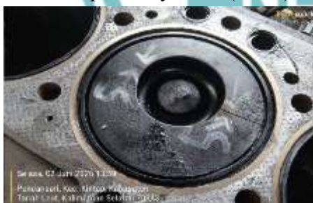
Detail liner cyl.no.5 (crack)
