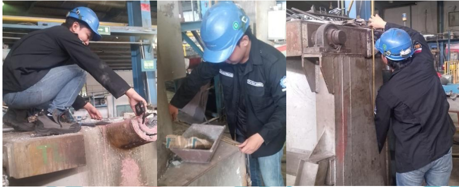
Gambar 3. 4 Pengukuran Geometri Melting Furnace
