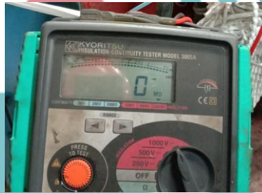
Gambar 4 5 Insulation Test indikasi Short to Ground
