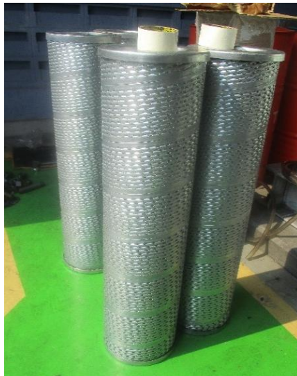
Gambar 6. Oil Separator Baru
