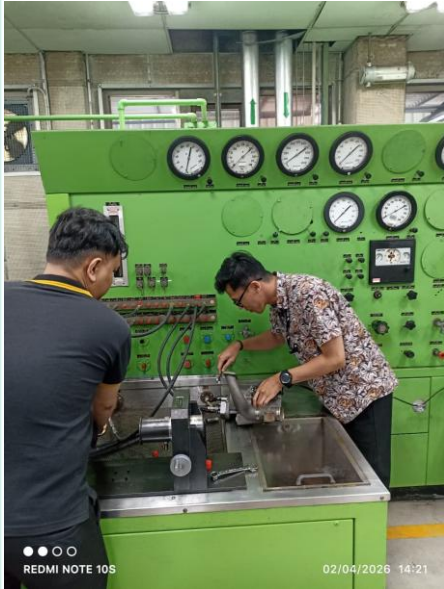
Lampiran 1. 1 Dokumentasi Fuel Leakage Test
