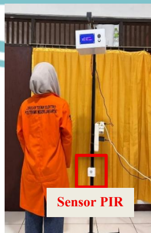
Gambar 4.17 Set Up Pengujian Sensor PIR
