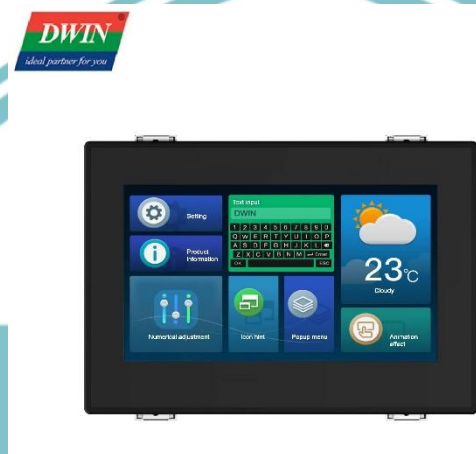
Gambar 2. 13 HMI DWIN DMG80480C070_15WTR 7 Inch
