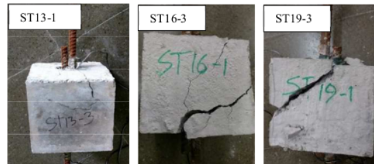
Fig. 8 The splitting failure pattern of fishbone rib bars specimen (ST)
