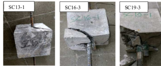
Fig. 7 The splitting failure pattern of slope rib bars specimen (SC)
