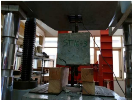
Fig. 4 The setting of pullout testing using UTM
