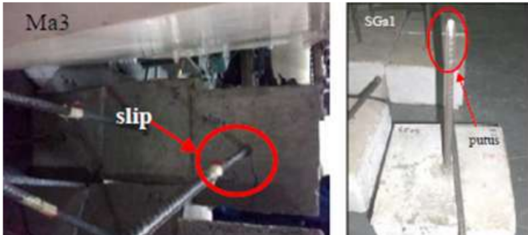
Figure 4. Damage to Specimen as the result of Ma and Sga Experiments
