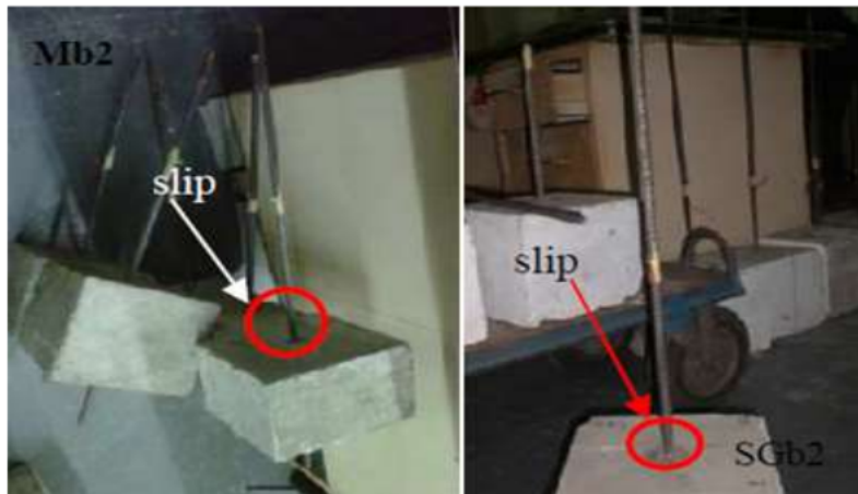
Figure 6. Damage to 160mm (Mb) and Sikagrout Id 160mm (Sgb) Monolithic specimens
