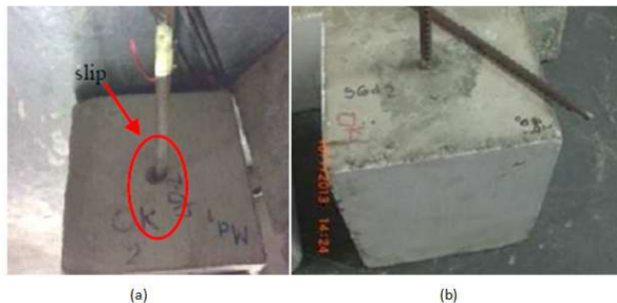
Figure 10. Damages to Monolith Id 260mm (Md) and Sikagrout Id 200mm (Sgd) specimens
