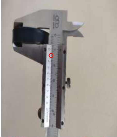
Pengukuran Groove Axial Width Seal U-Cup (10,1 mm)
