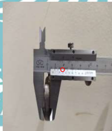
Pengukuran Groove Axial Diameter Seal Lip-Type (7,3 mm)
