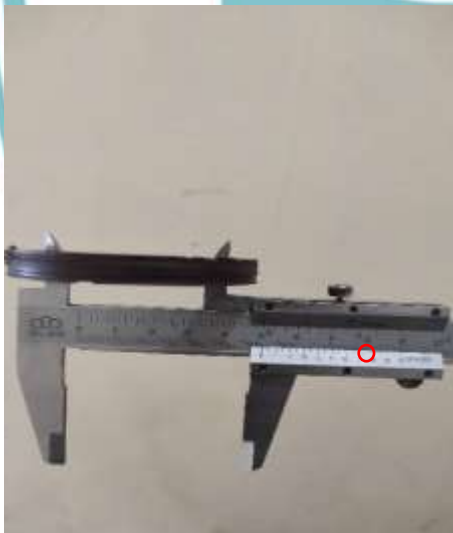
Pengukuran Groove Diameter Seal Piston (50,75 mm)
