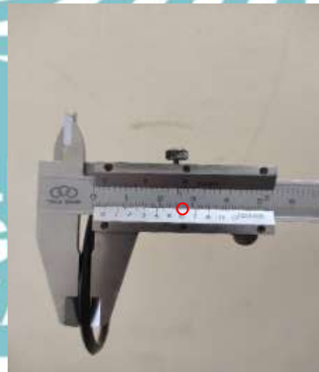
Pengukuran Cross Section Diameter Seal O-Ring 1 (3,6 mm)
