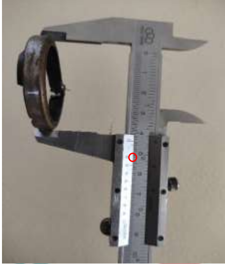
Pengukuran Groove Diameter Seal Lip-Type (44,2 mm)
