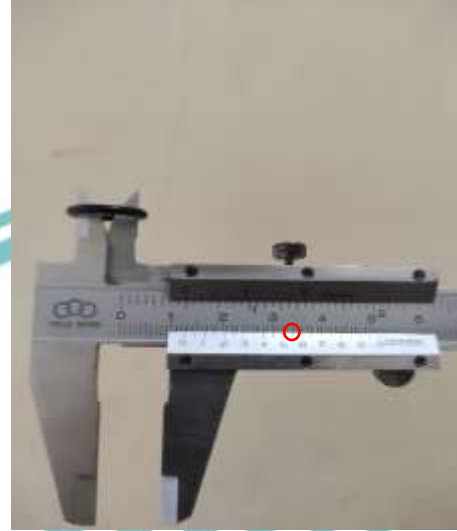
Pengukuran O-Ring Inside Diameter 1 Seal O-Ring 3 (12,55 mm)
