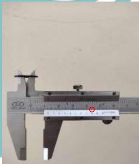
Pengukuran O-Ring Inside Diameter 2 Seal O-Ring 4 (12,8 mm)
