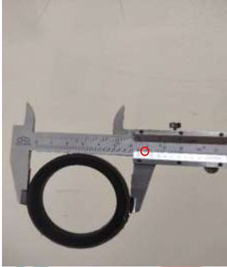
Pengukuran Bore Diameter Seal Piston (65,1 mm)
