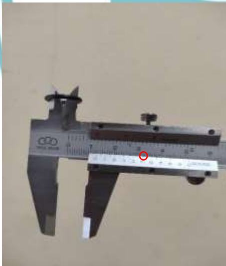
Pengukuran O-Ring Inside Diameter 2 Seal O-Ring 3 (12,5 mm)
