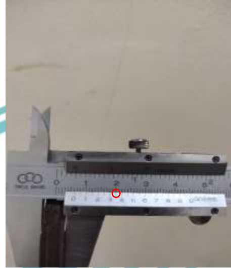
Pengukuran Groove Axial Width Seal Piston (6,35 mm)
