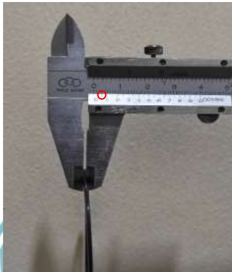
Pengukuran Axial Width Ring Backup (1,05 mm)
