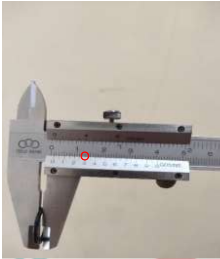
Pengukuran Cross Section Diameter 2 Seal O-Ring 4 (1,3 mm)
