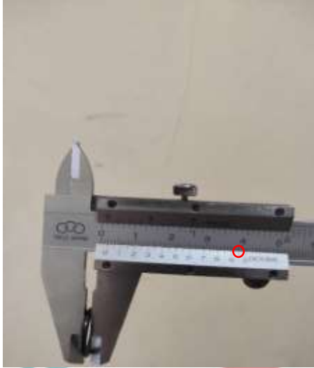
Pengukuran Cross Section Diameter 2 Seal O-Ring 3 (1,95 mm)
