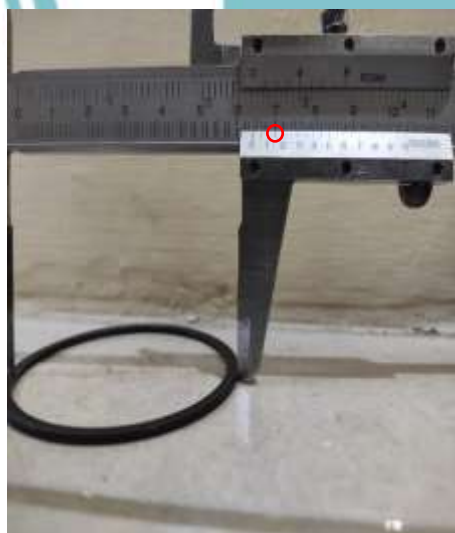
Pengukuran Outside Diameter Ring Backup (64,15 mm)
