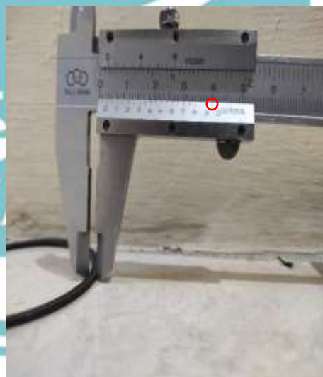
Pengukuran Radial Height Ring Backup (2,95 mm)
