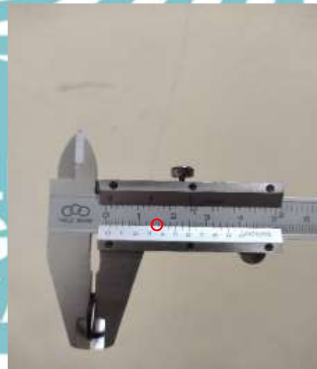
Pengukuran Cross Section Diameter 1 Seal O-Ring 4 (1,35 mm)
