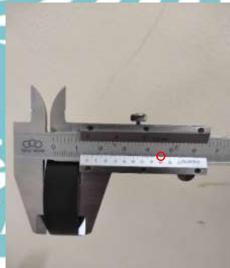
Pengukuran Groove Axial Width Ring Wear Piston (14,8 mm)
