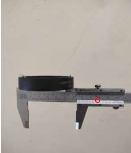
Pengukuran Groove Diameter Ring Wear Piston (57,55 mm)
