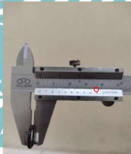
Pengukuran Cross Section Diameter 1 Seal O-Ring 3 (1,9 mm)
