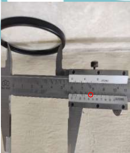
Pengukuran O-Ring Inside Diameter Seal O-Ring 2 (60,45 mm)
