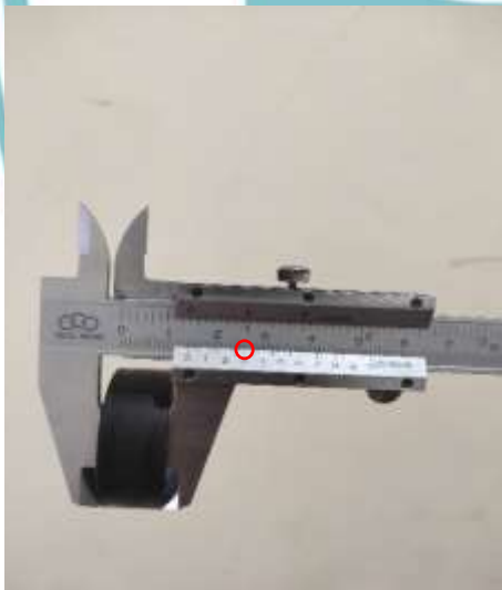
Pengukuran Groove Axial Width Ring Wear Head (14,3 mm)
