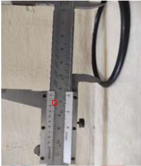
Pengukuran O-Ring Inside Diameter Seal O-Ring 1 (65,15 mm)
