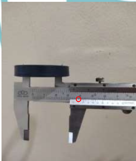
Pengukuran Rod Diameter Seal U-Cup (35,1 mm)
