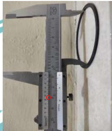
Pengukuran Inside Diameter Ring Backup (58,55 mm)
