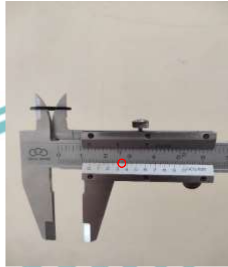
Pengukuran O-Ring Inside Diameter 1 Seal O-Ring 4 (13,5 mm)
