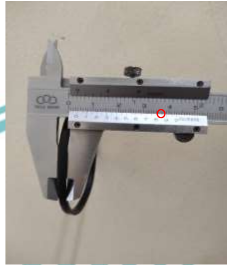
Pengukuran Cross Section Diameter Seal O-Ring 2 (3,85 mm)
