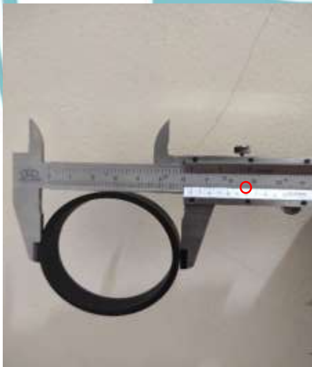
Pengukuran Bore Diameter Ring Wear Piston (63,6 mm)
