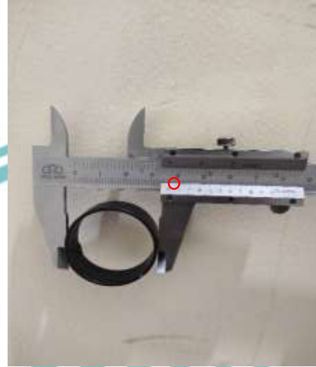
Pengukuran Bore Diameter Ring Wear Head (37,05 mm)
