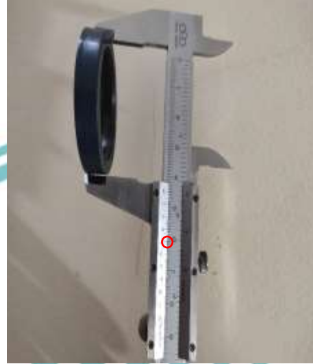
Pengukuran Groove Diameter Seal U-Cup (45,4 mm)
