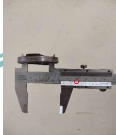
Pengukuran Rod Diameter Seal Lip-Type 36,35 mm)
