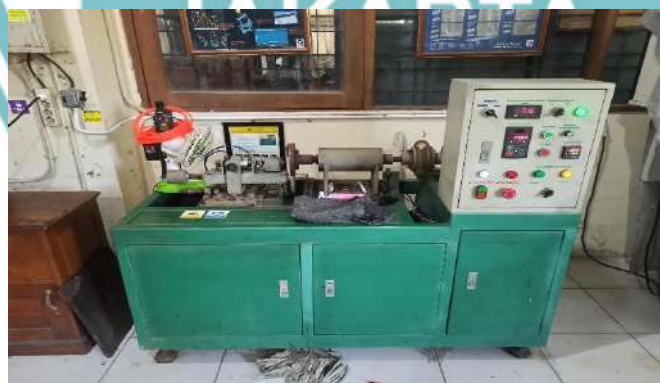
Alat Uji Tribometer Tipe Pin On Disk
