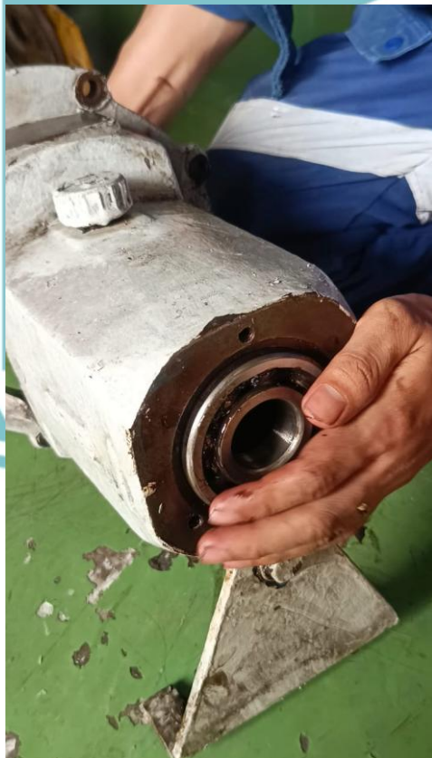
Lampiran 1. 3 Pemeriksaan Bearing dan Bearing Housing Pompa Sentrifugal
