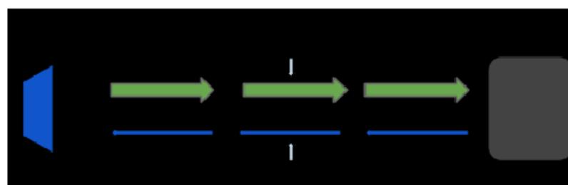
The sensor sends out a sound wave at a specific frequency. It then listens for that specific sound wave to bounce off of an object and come back (Figure 1). The sensor keeps track of the time between sending the sound wave and the sound wave returning. If you know how fast something is going and how long it is traveling you can find the distance traveled with equation 1.
