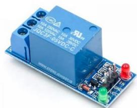
Gambar 2. 16 Relay 1 channel
