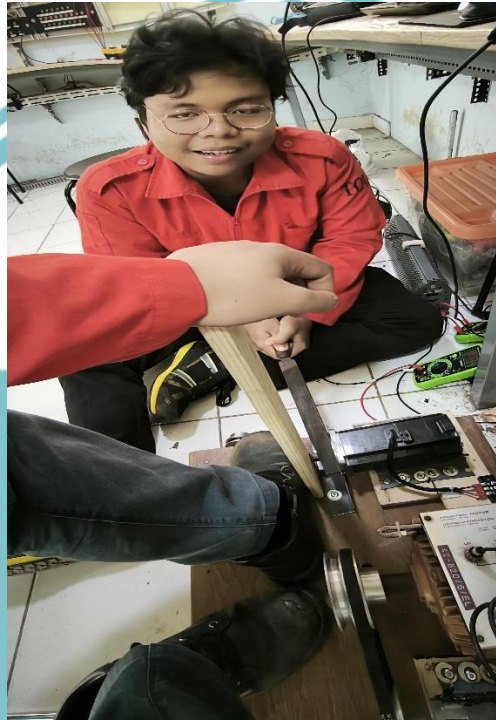
Pengikiran shaft generator
