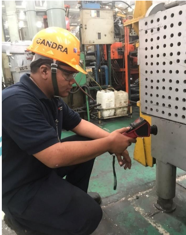
Lampiran 4 Pengecekan Loss Heat Keeping Furnace
