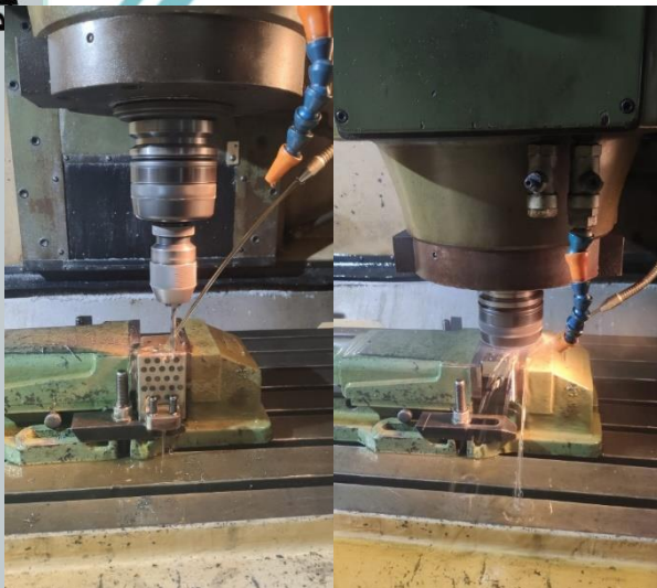
proses machining CNC 3A CAM dan Square Retainer.
