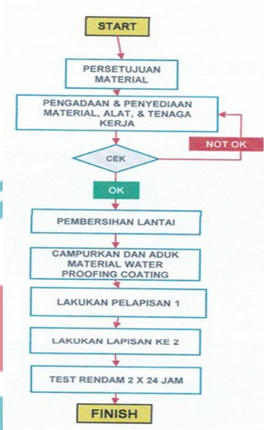
Gambar 3. 69 Flow Chart Pekerjaan Waterproofing
