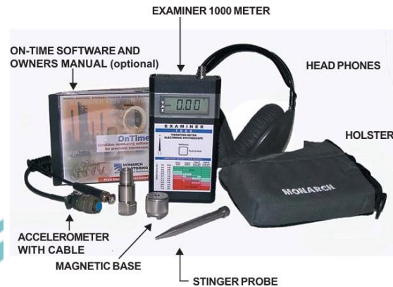
Gambar 4.8 Vibration Meter (Sumber: Monarch Instrument )
