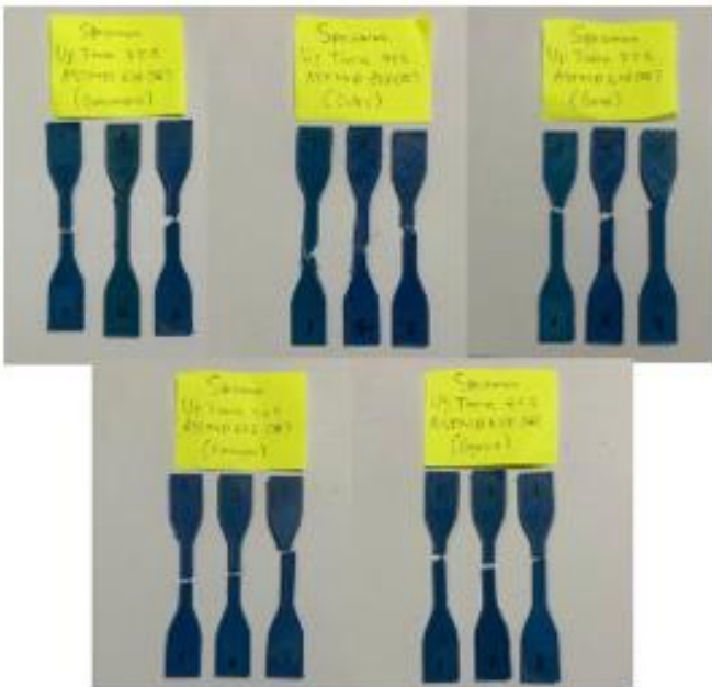
Hasil Patahan Uji Tarik Sampel 75%
