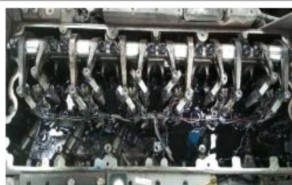
Picture of completed installation new injector
