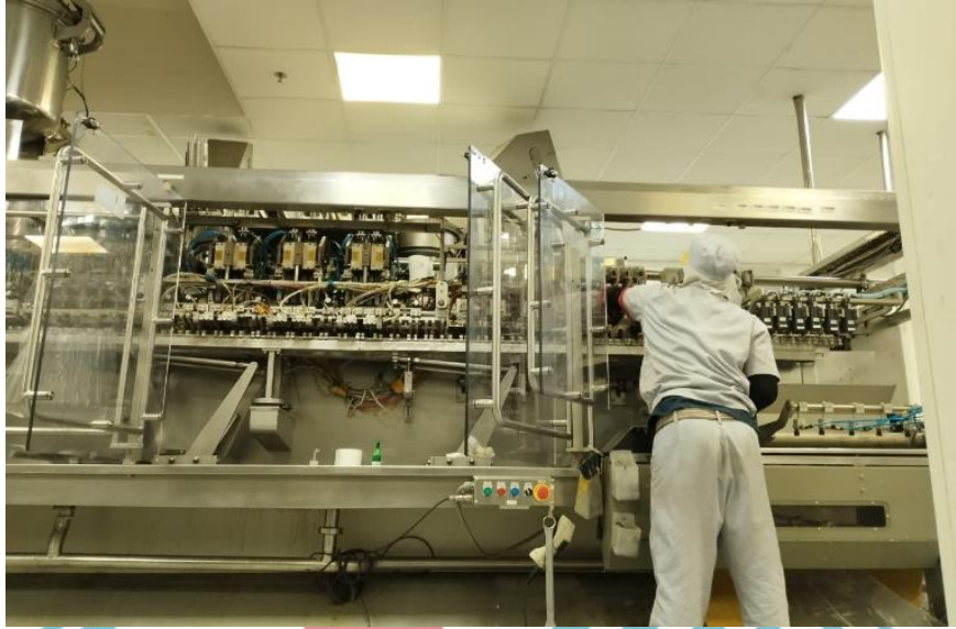
Bagian Cap Applicator sampai Pick and Place (Operator sedang membersihkan bagian Sealing )
