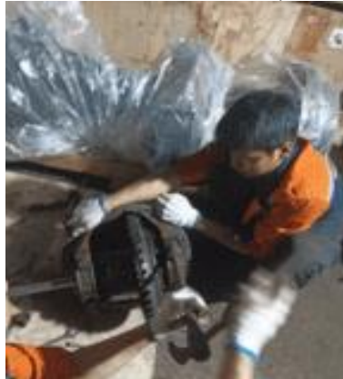
Gambar 8. Proses Pembongkaran Internal Differential
