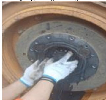
Gambar 3. Proses Pelepasan Axle Shaft
