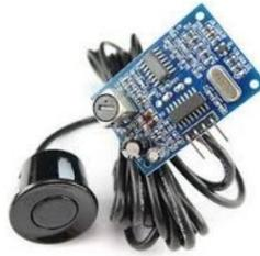
Gambar 2.3 Sensor Ultrasonik JSN SR04T
