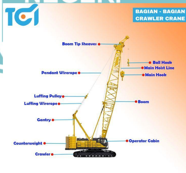
Gambar 2.4.2. 1 Bagian-bagian Crawler Crane
