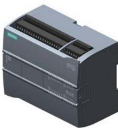
SIMATIC S7-1200, CPU 1215C, compact CPU, DC/DC/relay, 2 PROFINET ports, onboard I/O: 14 DI 24 V DC, 10 DO relay 2 A, 2 AI 0-10 V DC, 2 AO 0-20 mA DC, power supply: DC 20.4-28.8 V DC, program/data memory 200 KB
