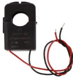
Fig 5 CT (Current Transformer) PZEM 004T
