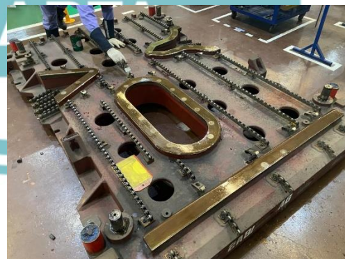
Preventive maintenance dies TAIL GATE FRAME
