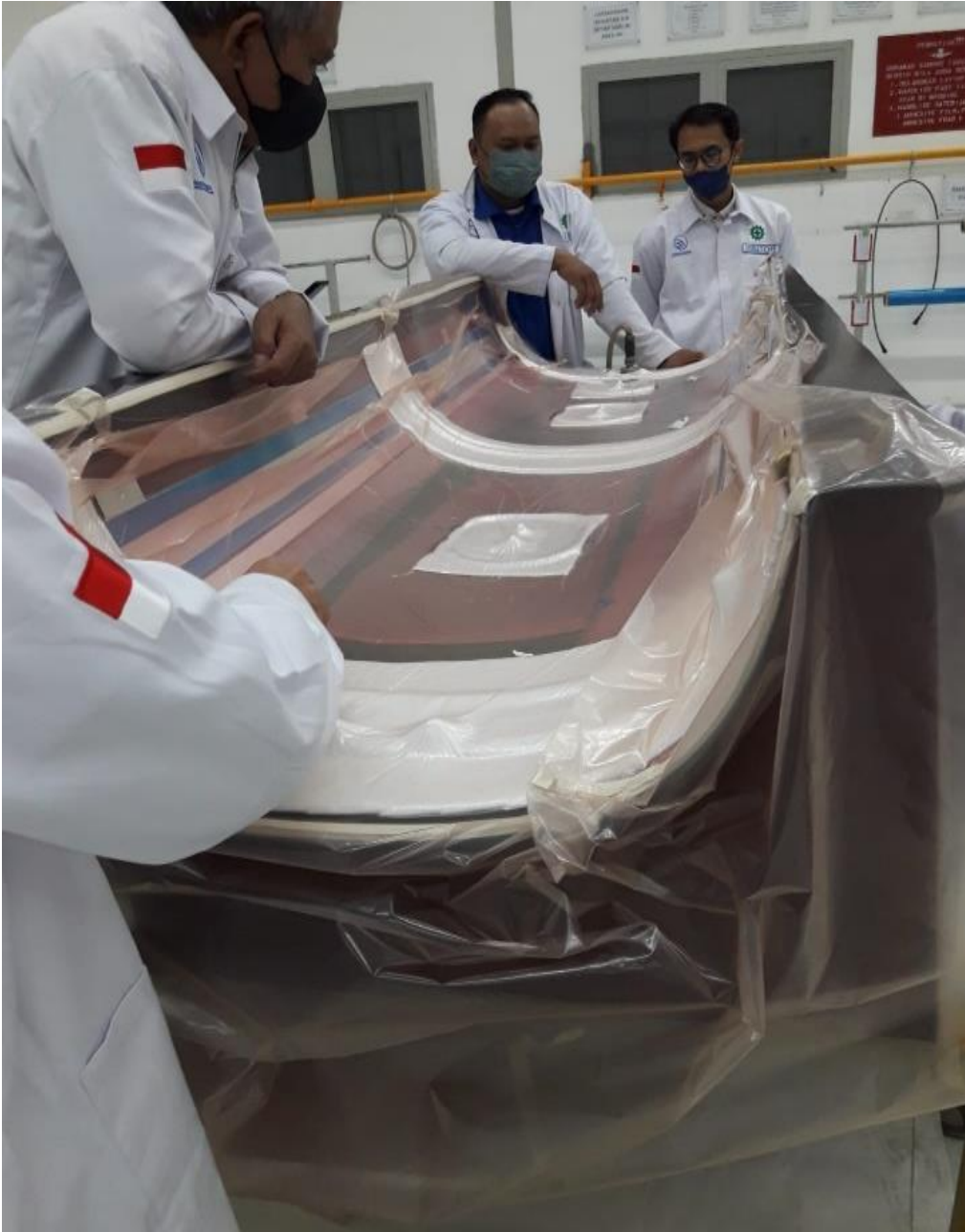
Lampiran 7. Dokumentasi Kegiatan Vacuum Bagging Panel Assy
