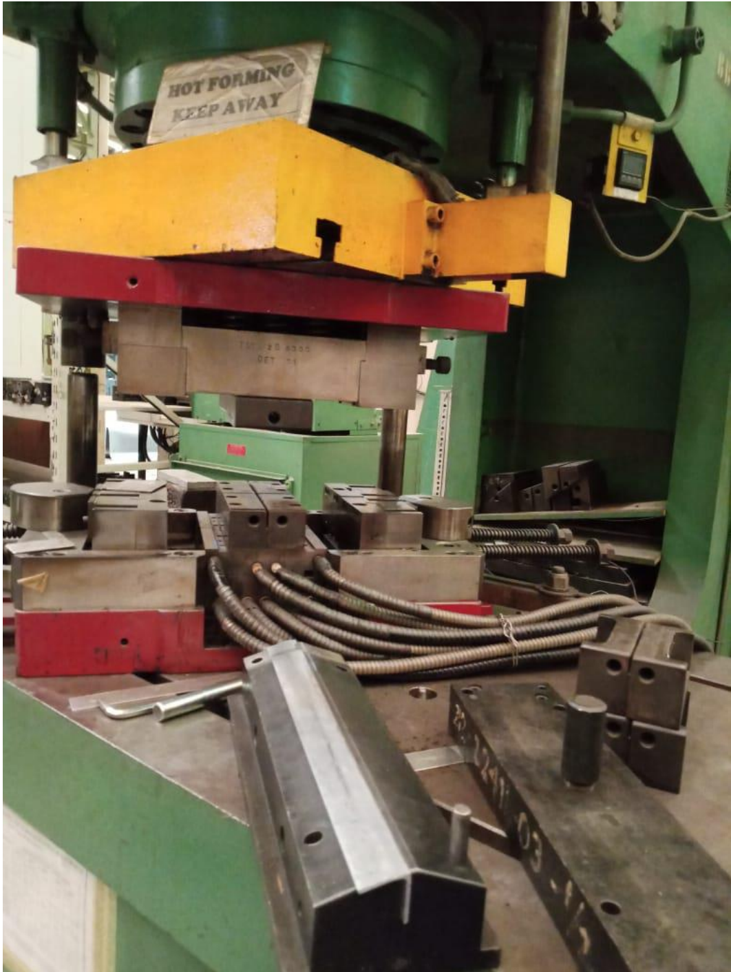
Lampiran 8. Hot Joggle Press Machine dan Dies
