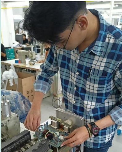
Pengecekan arus generator Ultrasonic sewing machine
