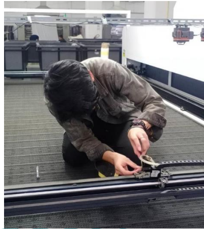
Kalibrasi head laser mesin laser cutting
