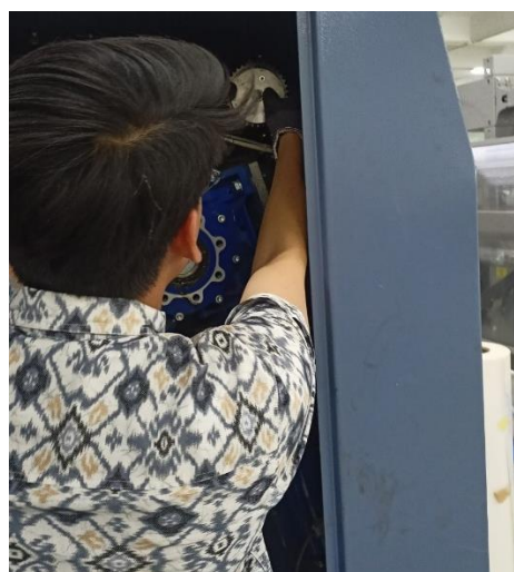
Pergantian gear mesin transmatic GFO 1067
