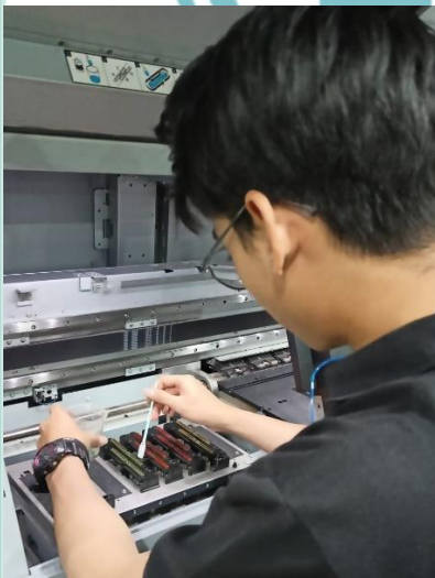
Cleaning manual printhead Epson F10030
