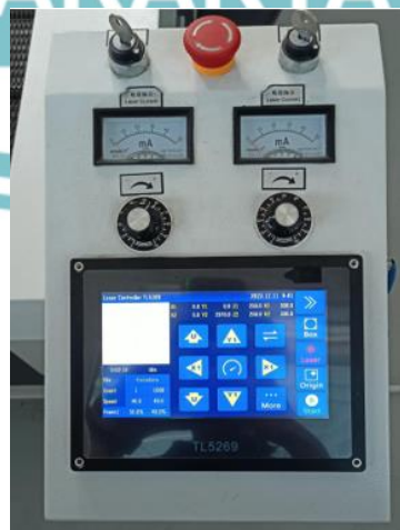
Gambar 3.16 Control Panel Laser Cutting Machine VK-3015
