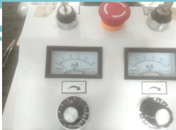
Gambar 3.24 Set-Up Ampere Laser
