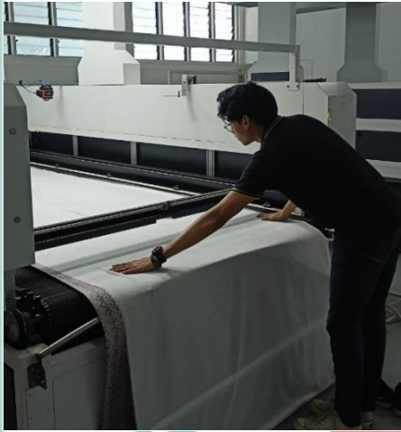
Set Up kain Laser Cutting machine
