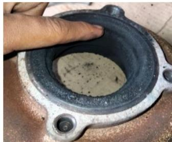
Gambar 11. Kebocoran turbocharger
