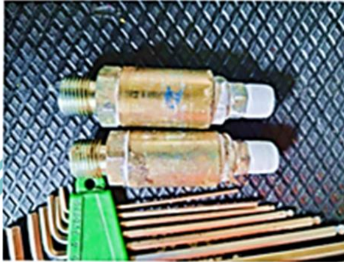
Lampiran 1 Aktifitas after re-sealing pada bagian connection pipe manifold
