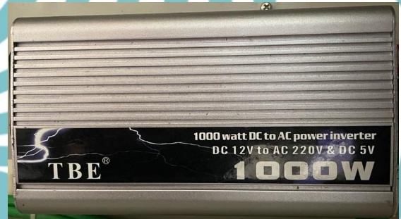
Inverter DC 12V to AC 220v 1000 W
