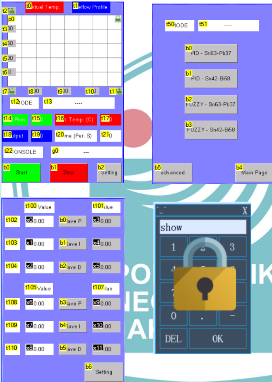
Gambar L.5 Design HMI Nextion Oven Reflow Sumber : Dokumentasi Pribadi
