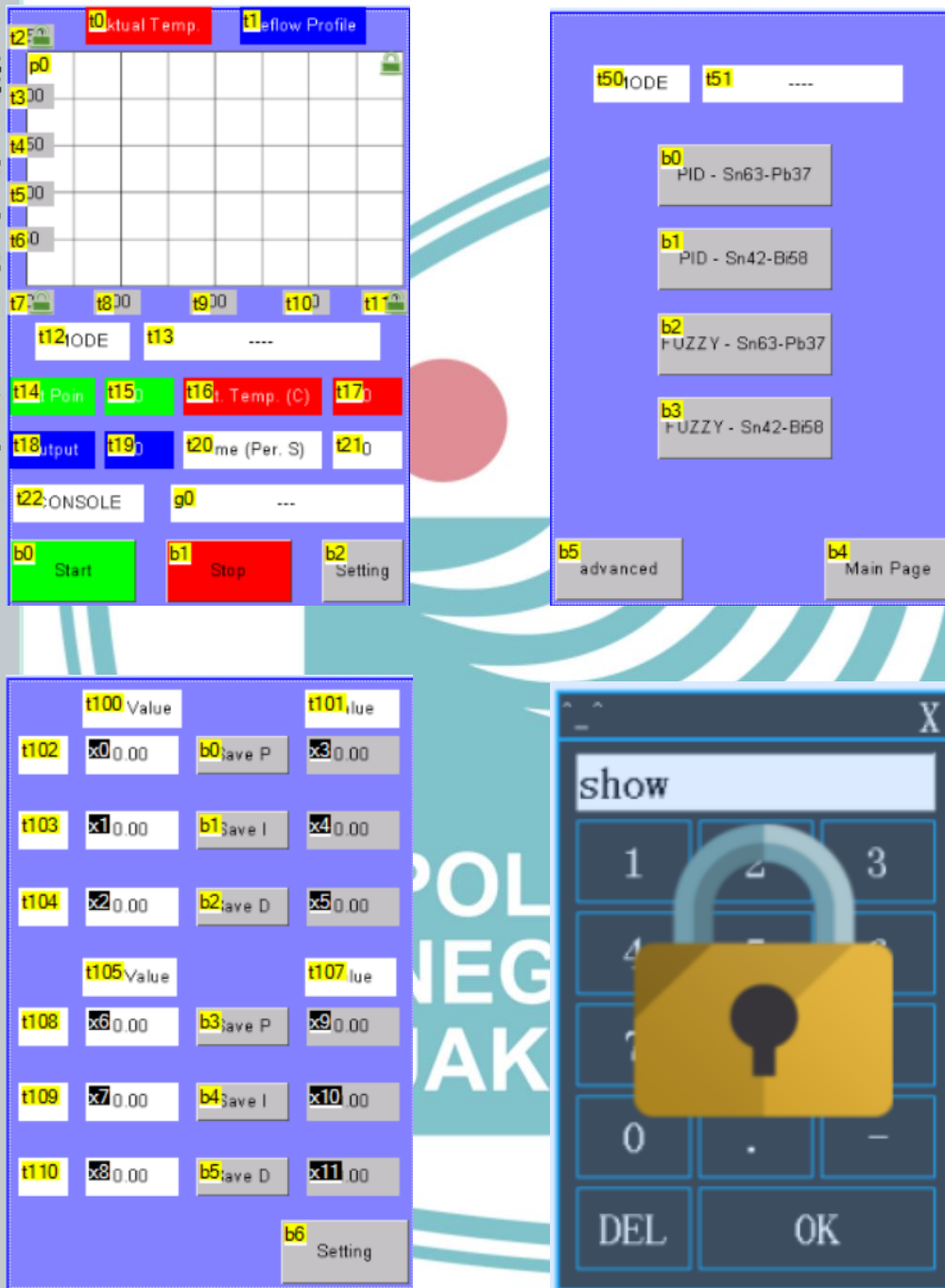
Gambar L.3 Design HMI Nestion Oven Reflow Sumber: Dokumen Pribadi
