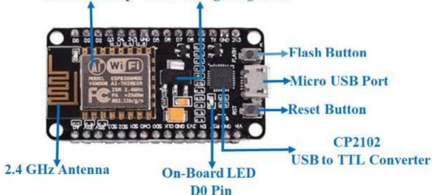
**NodeMCU Development Board Pinout Configuration**
